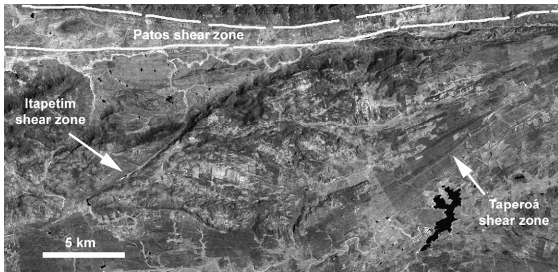
Fig. 4. Satellite image of the eastern termination of the Teixeira batholith (Pedra D'Água domain, see localization on Fig. 3). Note the sigma shape of the leucogranite sheets between Patos, Itapetim and Taperoá shear zone system.
